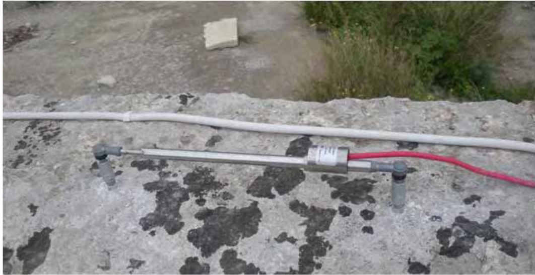
Figure 8.11: Picture of the dummy Gauge installed on an intact rock block (November, 2010).
