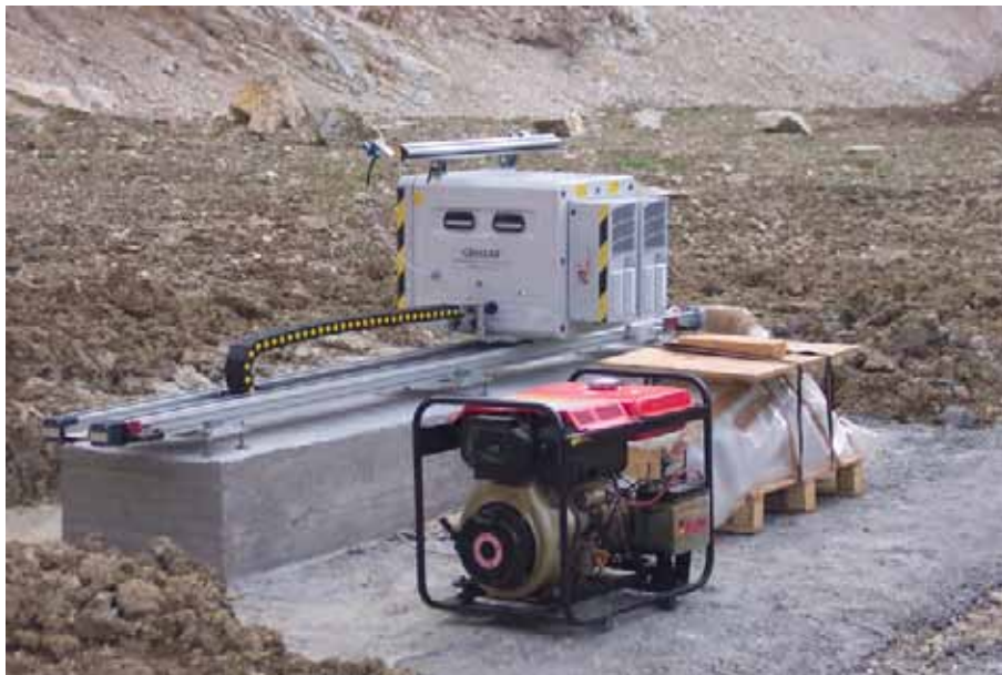
Figure 3.7: GBinSAR during monitoring activities at Torgiovannetto (April 2007).
