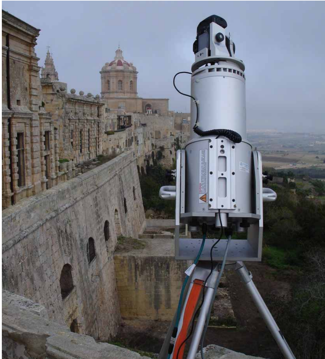
Figure 4.23: Laser Scanner Tool - LMS-Z420i during a Scanning on Mdina bastion walls (November, 2007).
