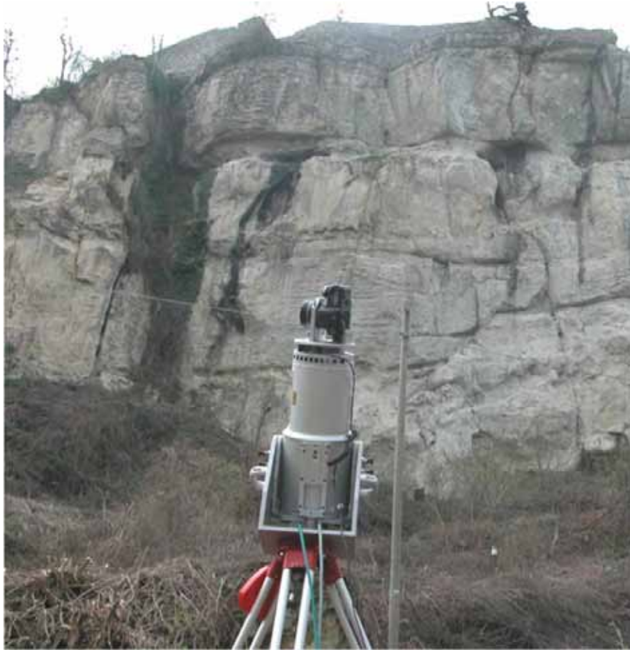
Figure 3.3: Laser Scanner Tool - LMS-Z420i Opposite to the Canossa wall cliff (Taken from [102]).
