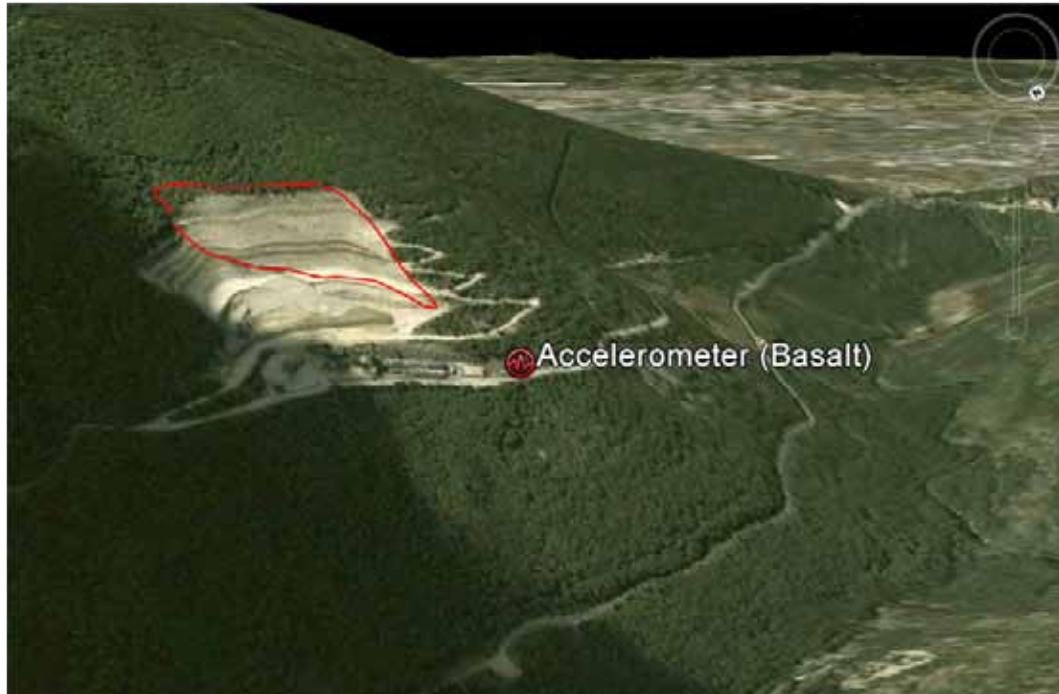
Figure 6.5: Bird View of Torgiovanetto landslide, accelerometer is installed at roadside (modified from [78]).
