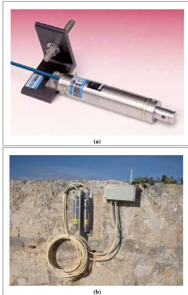
Figure 4.38: Vibrating Wire Tiltmeter “Geokon, Model 6350” installed on the Mdina walls (taken from [114]). a) Monoaxial configuration b) Biaxial configuration.
