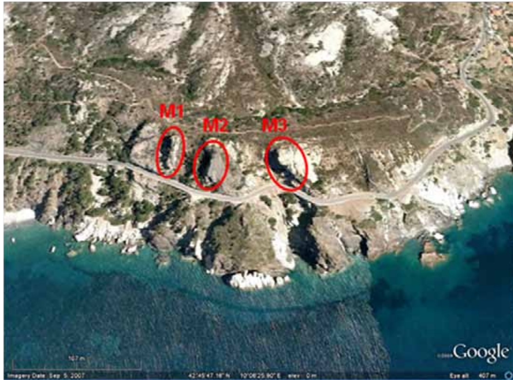
Figure 7.7: Portions of the rock mass, which overhang provincial road N° 25. Highlighted masses: mass 1 = M1, M2 = 2 mass, mass 3 = M3 (taken from [78]).
